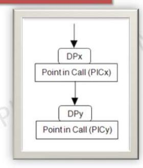
Detection Point (DP): smaller squares, indicates points where the need for IN functionality can be identified and the basic call handling suspended while the call control is transferred from basic call logic to the IN functionality in question.
